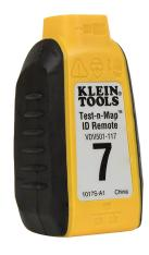
This replacement remote (#7) tests, maps and identifies a location in a single step, cutting testing and identification time in half. Test voice, data and video coax cable connections using Klein's Scout® Pro and Commander™ series of testers (sold separately). The remote is clearly numbered for fast, accurate identification. Up to eight individually numbered replacement remotes are available.
