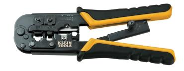
The all-in-one Ratcheting Modular Crimper/Stripper cuts, strips and crimps paired-conductor cables (round STP/UTP and flat-satin phone cables). Durably made from steel and finished in black oxide for high performance, it provides fast, reliable modular-crimp connector installation for voice- and data applications. Crimps 4, 6, and 8 position modular connectors (RJ22, RJ11/RJ12, and RJ45).
