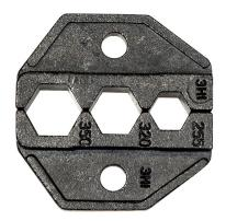
For use with Klein VDV200-010 Replacement Ratcheting Crimping Frame. Designed for Hex Crimp RG59/RG6 Coaxial Cable F-Connectors. Dimensions: 0.255 in. /0.320 in. /0.350 in. Durable construction. Crimp die for use with crimp connectors. Not for use with compression connectors.
