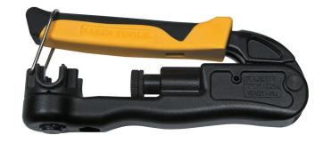
This Heavy-Duty, Multi-Connector Compression Crimper crimps most connectors to the majority of coaxial cables. for both inside (premises) and outside (utility) cabling. User-friendly gauge markings indicate correct plunger positions saving time and eliminating guesswork. The yellow and black contoured grips enhance comfort, visibility and allow quick identification. An integrated handle lock allows for easy storage on or off the jobsite.
