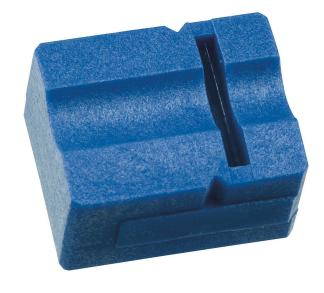
The Klein Tools Radial Stripper cartridge was designed to remove the outer jacket of twisted-pair cable without damaging the conductors. Specifically for use with Unshielded Twisted Pair (UTP) cables. Durable high-carbon steel cutting blades are ground and honed for long life. For use with Klein's Cartridge Radial Strippers.
