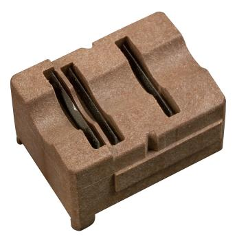
Cartridges made from glass filled polycarbonate for superior strength and extended durability. Pre-set cutting-blades for precise, accurate and efficient coaxial cable stripping. Durable high-carbon steel cutting blades are ground and honed for long life. Patented "V" notch eliminates scoring of the center conductor. Color coded for easy identification. Meets industry standards established by the SCTE (Society of Cable Telecommunication Engineers).
