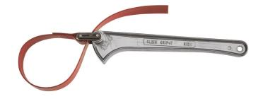
The Klein Tools 18-Inch Grip-It Strap Wrench is completely adjustable for tight-quarters tasks on polished, PVC and glass pipes, fittings, filters, conduit and shafts. The strap is urethane-coated to resist scratching or damaging surfaces and is attached to a lightweight I-beam handle. Also available in 12-Inch length (Cat. No. S12H).
