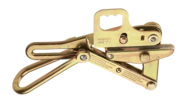
The Klein S1656-30H Chicago Grip-with Hot-Line Latch for Bare Conductors is for both bare and insulated conductors. The Klein S1656-30H Chicago Grip-with Hot-Line Latch for Bare Conductors may be placed on wire with hot-line stick. When stick is removed, latch closes automatically to guard against grip accidentally disengaging from wire.
