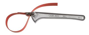
The Klein Tools 12-Inch Grip-It Strap Wrench is completely adjustable for tight-quarters tasks on polished, PVC and glass pipes, fittings, filters, conduit and shafts. The strap is urethane-coated to resist scratching or damaging surfaces and is attached to a lightweight I-beam handle. Also available in 18-Inch length (Cat. No. S18H).
