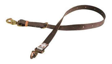
Klein's positioning straps work with Klein's climbing equipment for linemen. Made with exceptionally strong and long-lasting Klein-Kord, the straps are adjustable within a 2-Foot 3-Inch range. The drop-forged, single tongue adjustment buckle has a corrosion-resistant finish. Depending on the application, choose a positioning strap that allows you to work at arm's length from the pole or other positioning anchorage.
