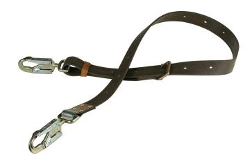
Klein's positioning straps work with Klein's climbing equipment for linemen. Made with exceptionally strong and long-lasting Klein-Kord, the straps are adjustable within a 1-Foot 10-Inch range. Features a Gard snap hook with 5000 lb. (2268 kg) gate strength. The drop-forged, single tongue adjustment buckle has a corrosion-resistant finish. Depending on the application, choose a positioning strap that allows you to work at arm's length from the pole or other positioning anchorage.
