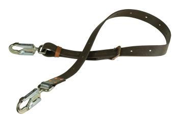
Klein's positioning straps work with Klein's climbing equipment for linemen. Made with exceptionally strong and long-lasting Klein-Kord, the straps are adjustable within a 2-Foor 6-Inch range. Features a Gard snap hook with 5000 lb. (2268 kg) gate strength. The drop-forged, single tongue adjustment buckle has a corrosion-resistant finish. Depending on the application, choose a positioning strap that allows you to work at arm's length from the pole or other positioning anchorage.
