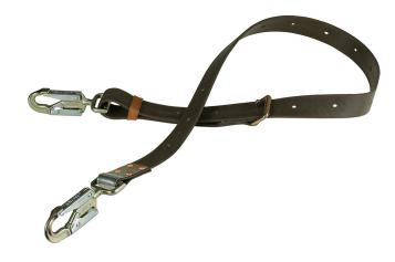
Klein's positioning straps work with Klein's climbing equipment for linemen. Made with exceptionally strong and long-lasting Klein-Kord, the straps are adjustable within a 2-Foot 3-Inch range. Features a Gard snap hook with 5000-Pound (2268 kg) gate strength. The drop-forged, single tongue adjustment buckle has a corrosion-resistant finish. Depending on the application, choose a positioning strap that allows you to work at arm's length from the pole or other positioning anchorage.
