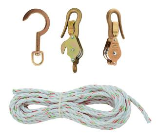
All Klein block and tackle use high-quality, 3/8-Inch (10 mm) diameter rope. Light, galvanized-steel shell blocks are fitted with snubbing hooks to hold the load. This package features two blocks with a swivel Klein hook Cat. No. 259 with a maximum safe load of 750-Pound (340 kg).
