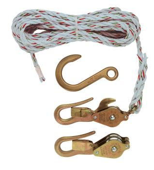
All Klein block and tackle use high-quality, 3/8-Inch (10 mm) diameter rope. Light, galvanized-steel shell blocks are fitted with snubbing hooks to hold the load. This package features two blocks with a forged standard Klein hook Cat. No. 258 with a maximum safe load is 750-pound (340 kg).
