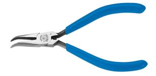
The 60-degree bent nose on these Midget Curved Chain-Nose pliers provide maximum work visibility in confined areas. This tool easily bends and forms fine wire. Polished inside jaws and radiused jaw edges prevent nicking wire while the curved handles provide greater tool control. Made of forged steel for maximum durability.
