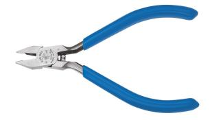
These 4-Inch Klein Tools Midget Electronics Diagonal Cutting Pliers have a semi-flush design to cut nickel ribbon wire. The nose tip is 1/32-Inch and the tip cutting knife is 3/16-Inch for precision in tight areas. Finally the pliers are forged from US steel and have induction hardened cutting knives and a hot-riveted joint for a long lasting smooth action.
