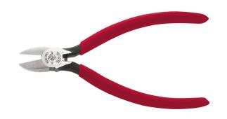
These Klein Tools Diagonal Cutting Pliers are designed with spring-loaded jaws for a self opening action. Their shortened jaws and beveled cutting edges permit close cutting in tight spaces. The induction hardened cutting knives made of US-forged steel, allow for a long lasting knife life.
