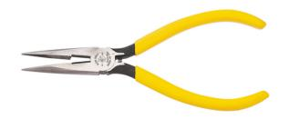
These Long-Nose Side-Cutters are spring-loaded for self-opening. The cutting knives are induction hardened for maximum life. Made of forged steel for durability with a long nose for grabbing and looping wire.
