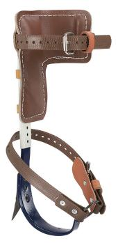
Klein's Pole Climber set includes the pads, steel sleeves, leg irons, gaffs, split rings and nylon calf and ankle straps. The secure sleeve and leg iron connections are adjustable. Contoured leg irons help position gaffs securely and comfortably. The replaceable gaffs firmly attach to the leg iron with a center pin and two TORX® screws. High-grade leather climber pads are cushioned for maximum comfort.
