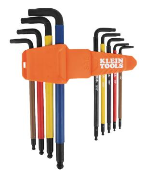
Klein Tools' 9-Key Color-Coded Hex Key Set conveniently consolidates the most popular SAE sizes into one compact caddy. The industrial strength, extended reach ball-end keys are optimal for working at angles up to 25 degrees. The round shanks with plastic sleeve provide enhanced comfort during prolonged use.
