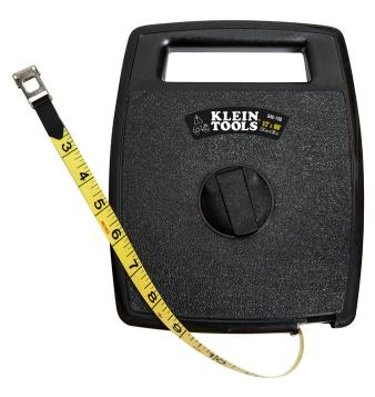
Klein Tools 100-Foot (30.48 m) Tape Measure is made from woven fiberglass tape with moisture-proof coating of polyvinyl chloride assures durability and protects against oil or chemicals. All metal parts are nickel plated for protection against rust. Tape line is graduated in feet and inches to 8ths.
