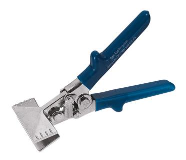
The Klein Tools Straight Hand Seamer helps make working with sheet metal, duct work, non-ferrous metals and tubing easy. This hand seamer is used for most general applications. The hand seamer has a compound-leverage design which helps give an accurate and powerful grip making tight seams. The steel jaws are places in 1/4-Inch increments for accurate bending measurements.
