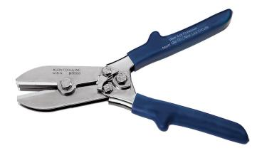
Klein Tools makes a wide variety of tools designed for sheet metal and HVAC applications, including this 5-Blade Crimper. With just the squeeze of a handle, this crimper produces factory-precision indentations in stove pipe and round duct. A combination of the compound-leverage mechanism, heavy-duty jaw/handle linkage, and closing stop provide easy operation and consistent crimps for virtually leak-proof connections.
