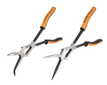
The Klein Tools 13-Inch Long Reach Pliers and Bent Nose Pliers are designed to improve access into tight spots across a variety of applications. The 2:1 double rivet design allows the jaws to open twice as wide as the handles, ensuring the ability to grip on a workpiece without obstruction. This 2-Piece set includes both straight and bent jaw pliers, with Klein's unique angled knurls to provide an extra grip that limits slippage.
