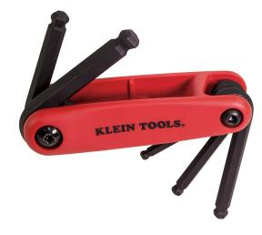
The Klein 70572 5-Metric Sizes Grip-It Hex Key Set has a ball design that allows for a thicker neck diameter which increases the torque capacity while maintaining operational angles to 25 percent. The keys are industrial strength, impact-resistant and tested for performance to below freezing temperatures. Key sizes are: 5mm, 6mm, 7mm, 8mm, 10mm, and the blades rotate independently up to 270 degrees.
