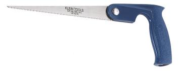
Magic-Slot design allows fast blade changing without removing thumbscrew. Strong, lightweight handle is contoured for comfort. High-quality carbon steel 8 in. blade has 10 teeth per inch for general-purpose use.
