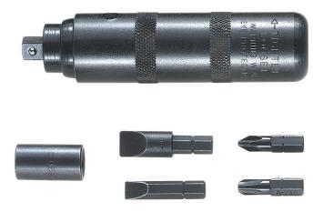
Klein Tools' Reversible Impact-Driver Set is a rugged, hand-impact driver designed to turn rusted, frozen, or other stubborn screws. The internal, springloaded, helical design transforms the impact of a hammer blow up to 200 ft.-lbs. of shock torque. It can also be used with 3/8-Inch square-drive impact sockets.
