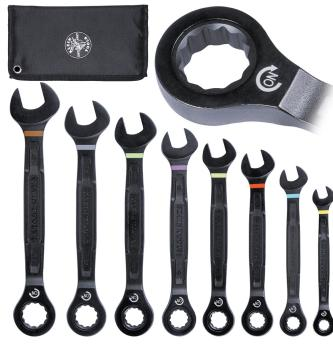
The Klein Tools Ratcheting Combination Set contains eight metric wrenches with color coded size markings to easily identify each tool. These wrenches are made from cold-forged steel alloy precision machining finish and black phosphate coating for long-lasting rust prevention. The 90-tooth ratchet mechanism minimizes the return angle for maximum access.
