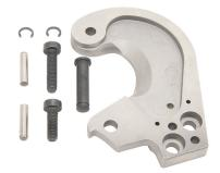
Replacement blade set for use with Klein's Cat. No. 63607 Ratcheting Cable Cutter (Pre-2017 Edition). Forged, heat-treated, shear-type cutting blades are made of hardened steel for sharpness and long life. Cuts up to 336 MCM ACSR, 400 MCM copper and 600 MCM aluminum.
