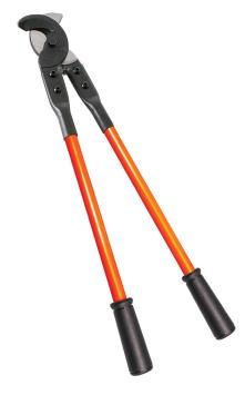
Klein Tools Standard Cable Cutters are lightweight, yet efficient. They feature replaceable hook-jaw blades that grab and hold cable while the shear-cutting action makes clean cuts. The jaws are made of forged tool steel with a black-oxide finish for long life. The exceptionally strong fiberglass handles have heavy vinyl grips for added comfort and slip resistance.
