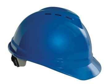
The lightweight design provides added comfort on the job. The built-in vents let cool air flow in while warm air flows out. The Glareguard™ under the brim reduces reflective glare. Lateral contours above the ear allows for easy integration of hearing protection. This style features a plain front with the Klein Tools Logo and American Flag on the back.
