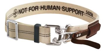
Klein's Tool Belt features a forged, quick-release buckle for emergency situations where the user has to quickly disengage the belt (e.g. working over water or in grain elevators). Belt is made of a mildew-resistant blend of cotton/polyester webbing for comfort and strength. Comfort and safety all in one.
