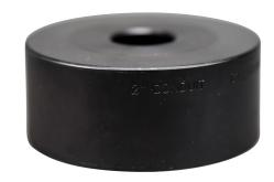
Klein 2.416 Knockout Die allows you to easily punch holes for 2-Inch EMT conduit. Has a maximum capacity of 10 gauge mild steel. Cuts aluminum, fiberglass and plastic as well.
