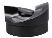
Easily punch holes for1-1/2-Inch EMT conduit. Has a maximum capacity of 10 gauge mild steel. Cuts aluminum, fiberglass and plastic as well. Optimized design reduces wrench effort. Slugs are split inside for easy removal.
