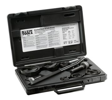
The Klein Tools knockout punch set with wrench is a great solution for electrical professionals and enthusiasts alike. This set features a 1-Inch ratcheting wrench, knockout punches, dies, and draw studs for conduit sizes ranging from 1/2 to 2-Inch. With a cutting capacity of 10 gauge mild steel, it also handles materials like aluminum, fiberglass, and plastic as well. Built for precision and efficiency, this kit ensures clean and accurate hole punches while splitting slugs for easy removal.
