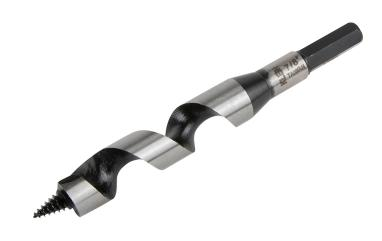
The deep, open-throat design of the Ship Auger bit clears chips for faster, cleaner cuts. The shank is 7/16-Inch hex to fit 1/2-Inch (13 mm) and larger three-jaw chucks. Used for heavy construction and repair work in mines, on docks and bridges as well as electrical work.
