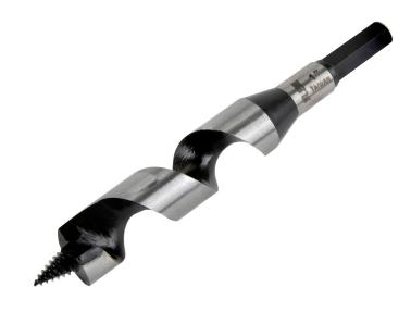
The deep, open-throat design of the Ship Auger bit clears chips for faster, cleaner cuts. The shank is 7/16-Inch hex to fit 1/2-Inch (13 mm) and larger three-jaw chucks. Used for heavy construction and repair work in mines, on docks and bridges as well as electrical work.
