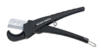
The Klein Tools 3/4 in. PVC Cutters are ideal for cleanly cutting schedule 40 PVC piping. They are crafted with steel for strength and feature 4 in. handles and a reversible blade for a longer cutting life. The cutters work well for cutting schedule 40 PVC piping with diameters up to 3/4 in. and flexible piping with diameters up to 1-3/8 in.
