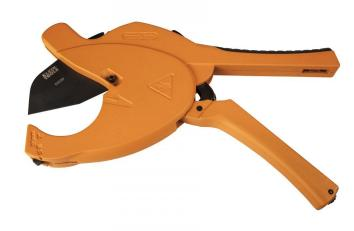
The Klein Tools ratcheting PCV cutter cuts white and gray 1/2-Inch to 2-1/2-Inch white and gray schedule 40 and 80 PVC. The ratcheting action allows for easy, one-handed cutting and blade release. Lightweight, comfortable handle reduces hand fatigue.
