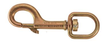
The Klein Tools 750-pound 1/2-Inch Steel Swivel Hook with Plunger Latch is made from forged steel. It can hold up to 750 pounds. The swivel action of the clevis allows smooth rotation to help prevent accidental fouling into secondary wires.
