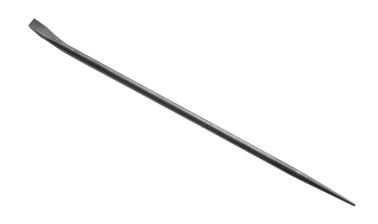
Klein Tools Round Connecting Bars are designed so they provide extra-leverage when positioning steel members and aligning bolt holes. Round bars are made of hardened steel for durability and long life. The chisel-end is at a 15-Degree angle to give greater leverage.
