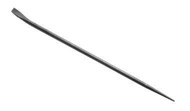
Klein Tools Round Connecting Bars are designed so they provide extra-leverage when positioning steel members and aligning bolt holes. Round bars are made of hardened steel for durability and long life. The chisel-end is at a 15-Degree angle to give greater leverage.
