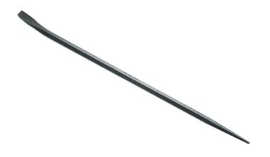
Klein Tools Hex Connecting Bars are designed so they provide extra-leverage when positioning steel members and aligning bolt holes. Hex bars are made of hardened steel for durability and long life. The chisel-end is at a 15-degree angle to give greater leverage.
