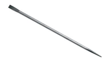
Klein Tools Hex Bars are designed so they provide extra-leverage when positioning steel members and aligning bolt holes. Hex bars are made of hardened steel for durability and long life. These forged fit-up bars are pointed on one end for versatility.
