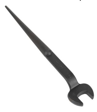
Forged from select alloy steel, Klein Tools' 1-1/8-Inch Nominal Opening Spud Wrench is designed to withstand high-leverage and heavy loads. For use with 3/4-Inch bolts and U.S. regular nut types, the extra-duty head area provides maximum strength and durability. Plus, the continuous taper of the handle makes it easy to line up bolt holes.
