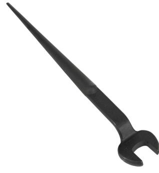
Forged from select alloy steel, the Klein Tools 1-Inch Nominal Opening Spud Wrench is designed to withstand high-leverage and heavy loads. It's designed for use with 5/8-Inch bolts and U.S. regular nut types. The extra-duty head area gives maximum strength and durability. Plus, the continuous taper of the handle makes it easy to line up bolt holes.
