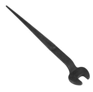
Forged from select alloy steel, the Klein Tools 13/16-Inch Nominal Opening Spud Wrench is designed to withstand high-leverage and heavy loads. It's designed for use with 1/2-Inch bolts and U.S. regular nut types. The extra-duty head area gives maximum strength and durability. Plus, the continuous taper of the handle makes it easy to line up bolt holes.
