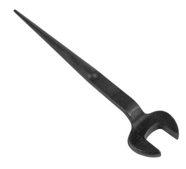
Forged from select alloy steel, the Klein Tools 1-5/8-Inch Nominal Opening Spud Wrench is designed to withstand high-leverage and heavy loads. It's designed for use with 1-Inch bolts and utility nut types. The extra-duty head area gives maximum strength and durability. Plus, the continuous taper of the handle makes it easy to line up bolt holes.
