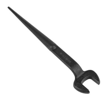
Forged from select alloy steel, the Klein Tools 1-7/16-Inch Nominal Opening Spud Wrench is designed to withstand high-leverage and heavy loads. It's designed for use with 7/8-Inch bolts and utility nut types. The extra-duty head area gives maximum strength and durability. Plus, the continuous taper of the handle makes it easy to line up bolt holes.
